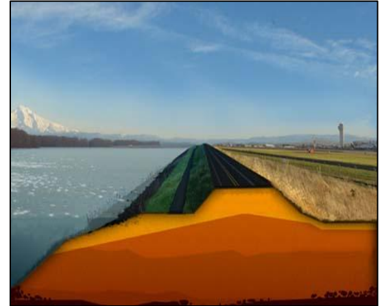
Diagram of a levee illustrating the original river bank (darkest orange at the bottom), the core of the levee (orange triangle in the middle), and additional material on top of the levee (yellow).
